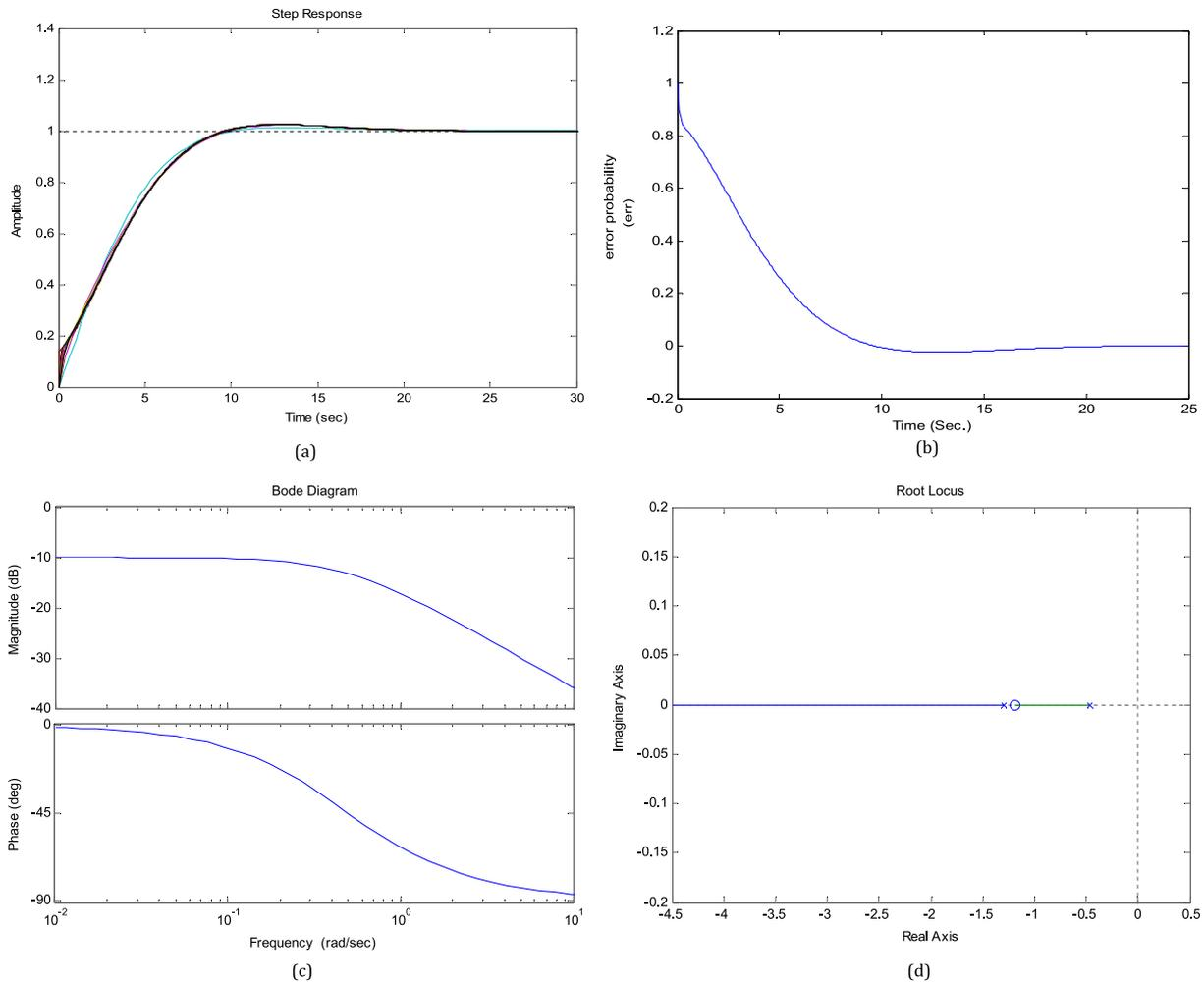
Fig. 4.3. System responses after tuning: (a) step response of prototype using filter; (b) error probability; (c) Bode plot; (d) root locus.
