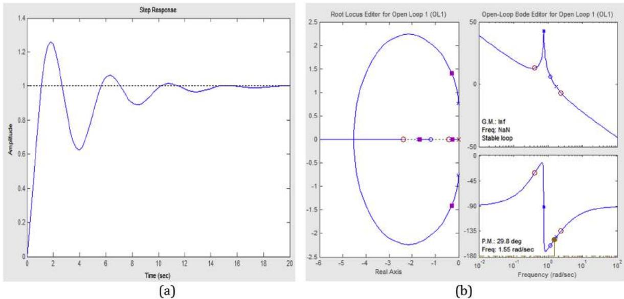
Fig. 4.4. System (a) step response; (b) root locus and bode plot after PID tuning.
