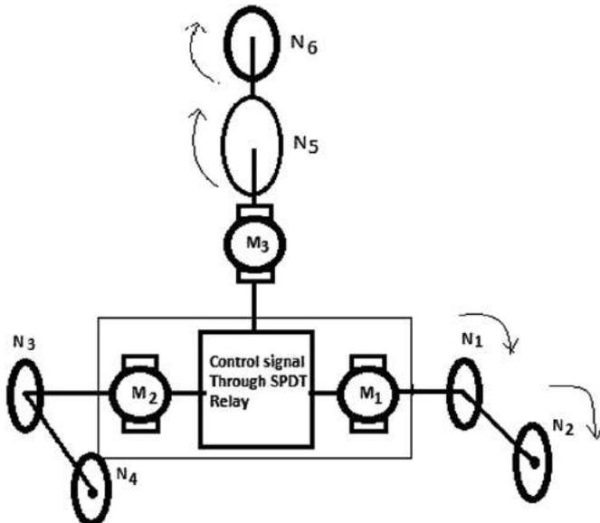
Fig. 3.4. Wheel rotation both for horizontal and vertical sections in prototype.
