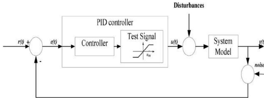
Fig. 3.1. Block diagram of control mechanism for prototype.
