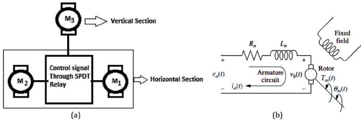
Fig. 3.3. (a) Block diagram representation of prototype motor utilization (b) Equivalent circuit of motor.
