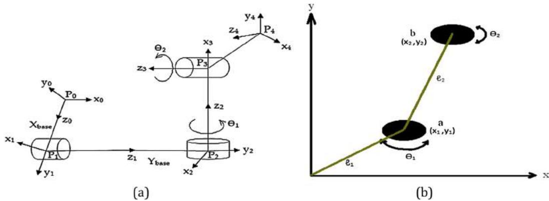
Fig. 2.2. (a) D–H frames for automation system. (b) Two DOF representation on  $x$  and  $y$  axes.
