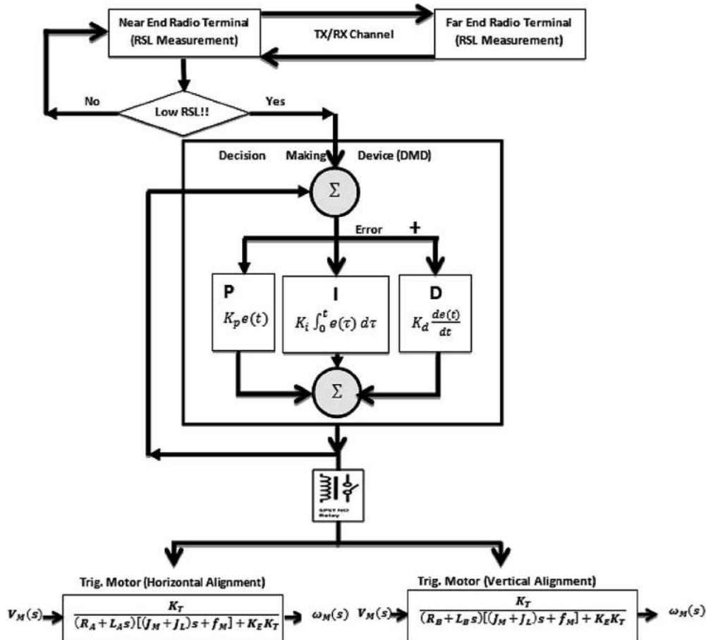
Fig. 3.2. Prototype analytical model for antenna realignment.
