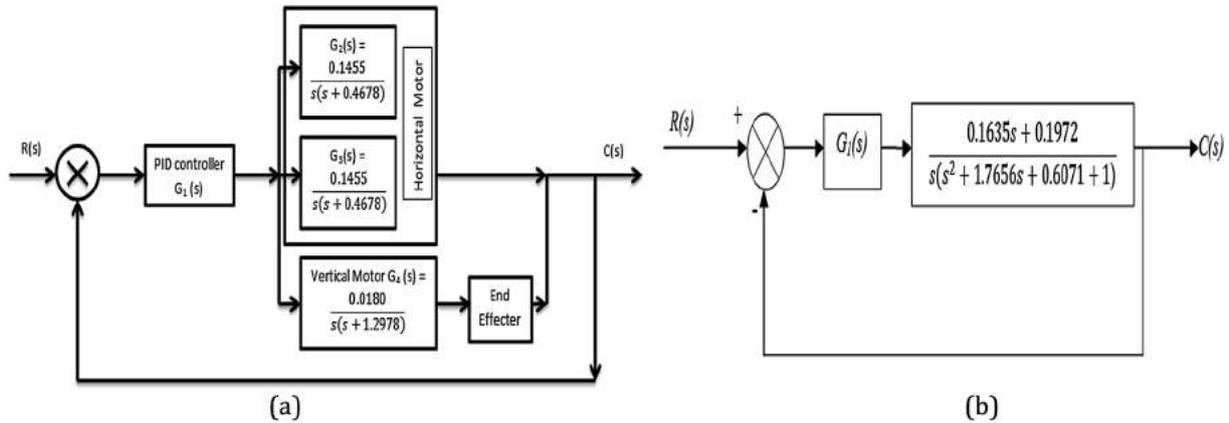
Fig. 3.5. Block diagram representation of prototype: (a) detail structure with transfer function; (b) reduced block.
