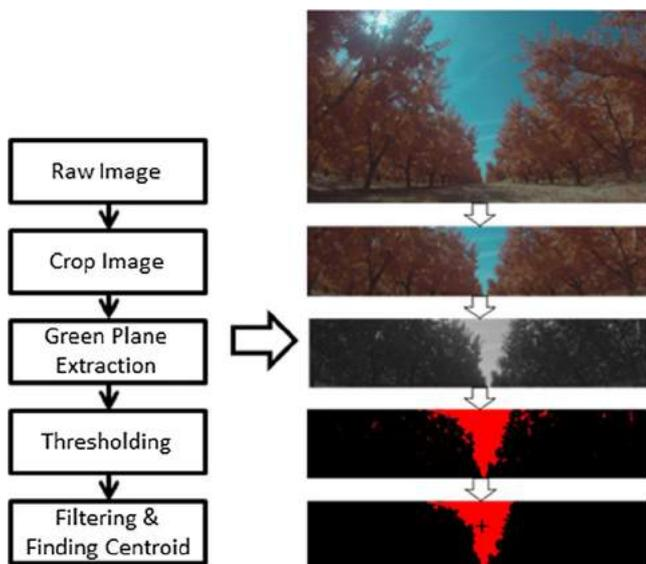
Fig. 5. Image processing algorithm for autonomous navigation.
