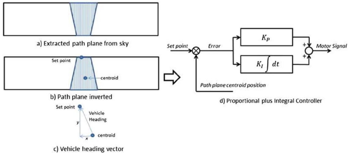
Fig. 6. Calculation of vehicle heading vector and PI controller of feedback system.
