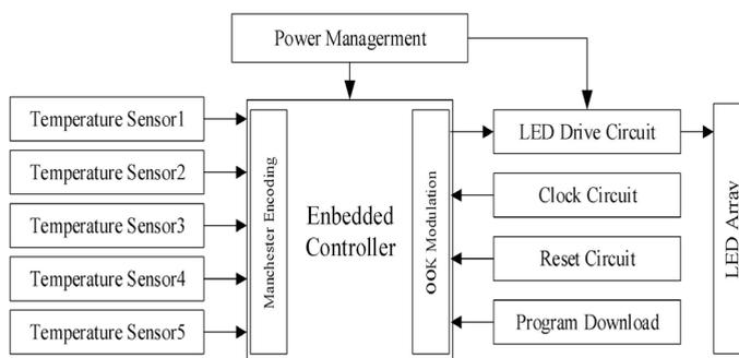
Fig. 1. The overall block diagram of acquisition device.
