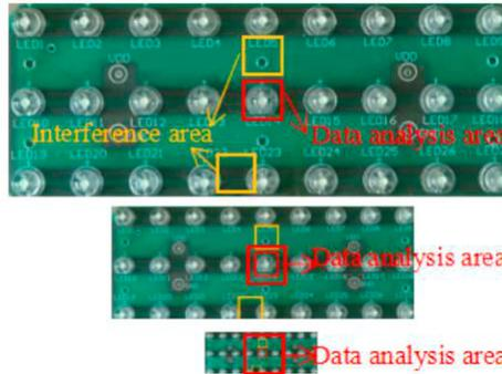
Fig. 11. Data analysis area of led panel.
