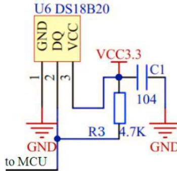
Fig. 2. The circuit of temperature sensor.
