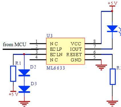
Fig. 4. The circuit of LED driver.
